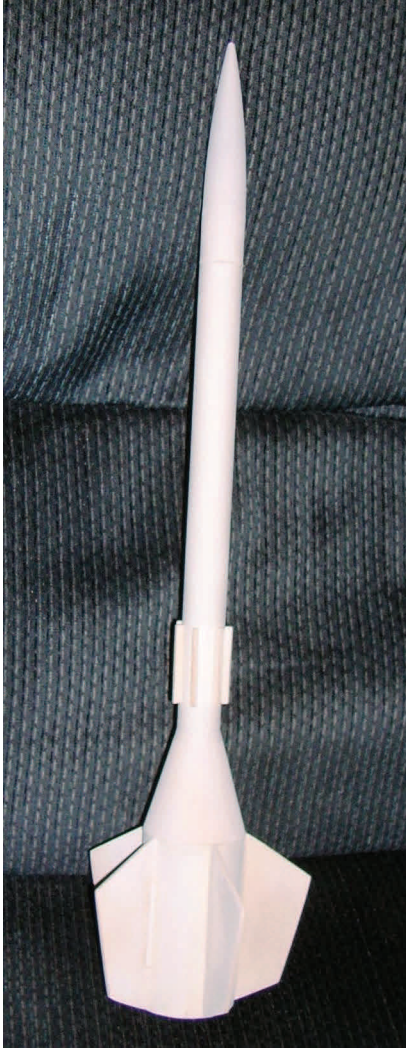
Finished filled and sealed, without paint
